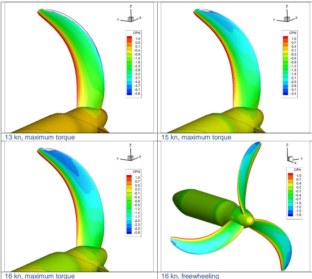
**Figure 5-2:** Computed pressure distributions (contour) and cavitation extent (white shade).
