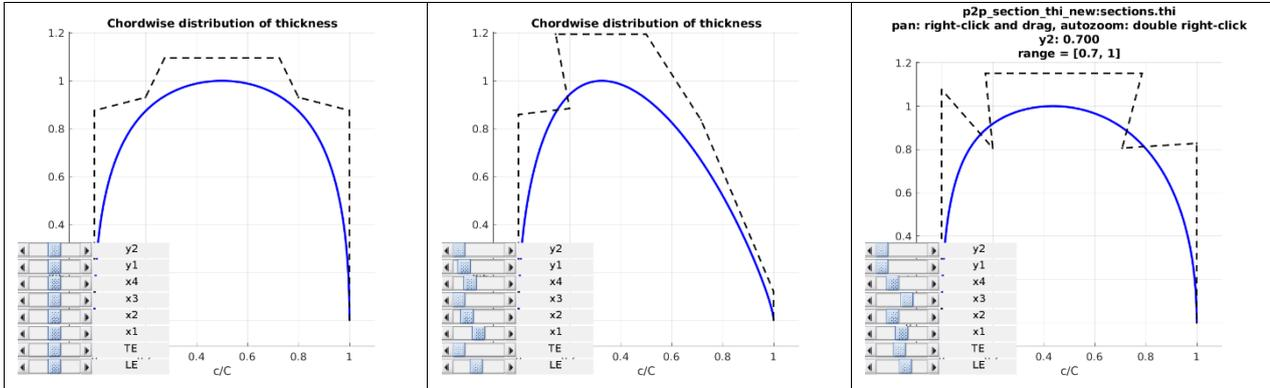
**Figure 4-3:** *Bezier parametrisation of the chordwise distribution of thickness (3 variations shown).*
