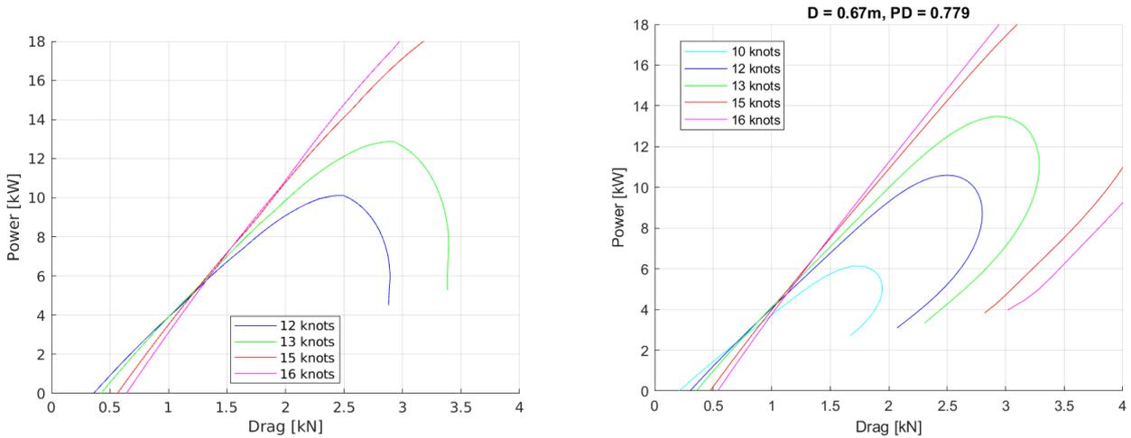
**Figure 5-7:** Propeller power versus total drag, computation (left) and measurements (right)
