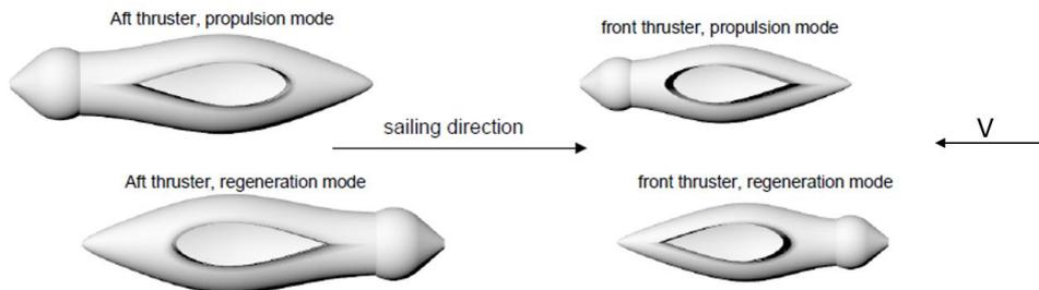
Figure 4-6: Modes of operation for front and aft thruster
