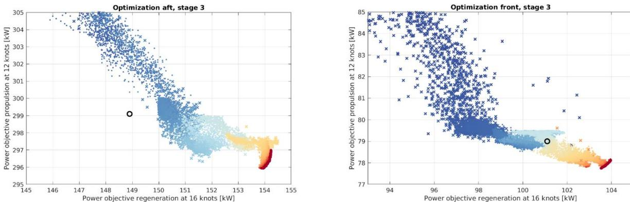
**Figure 4-4:** *Optimization results, converging from blue to red. The black circle is the reference design.*
