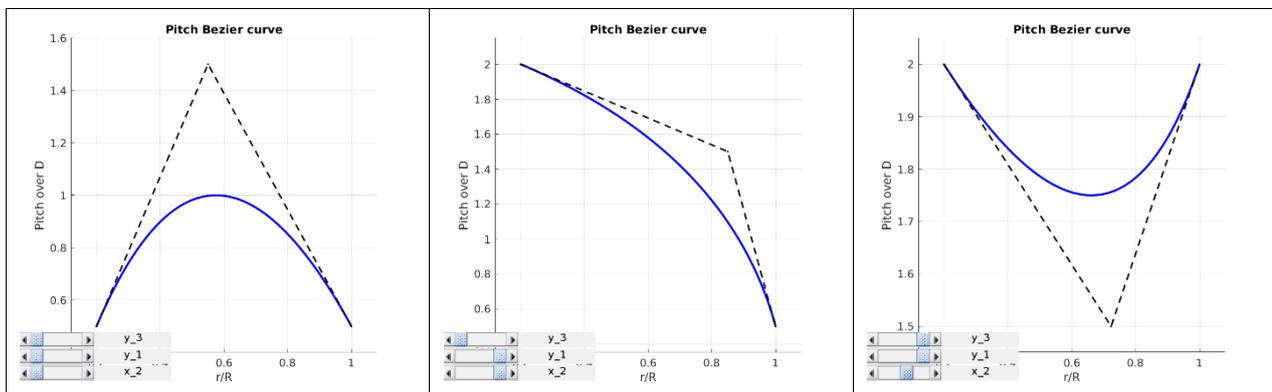
Figure 4-1: Bezier parametrisation of the radial pitch distribution (3 variations shown).
