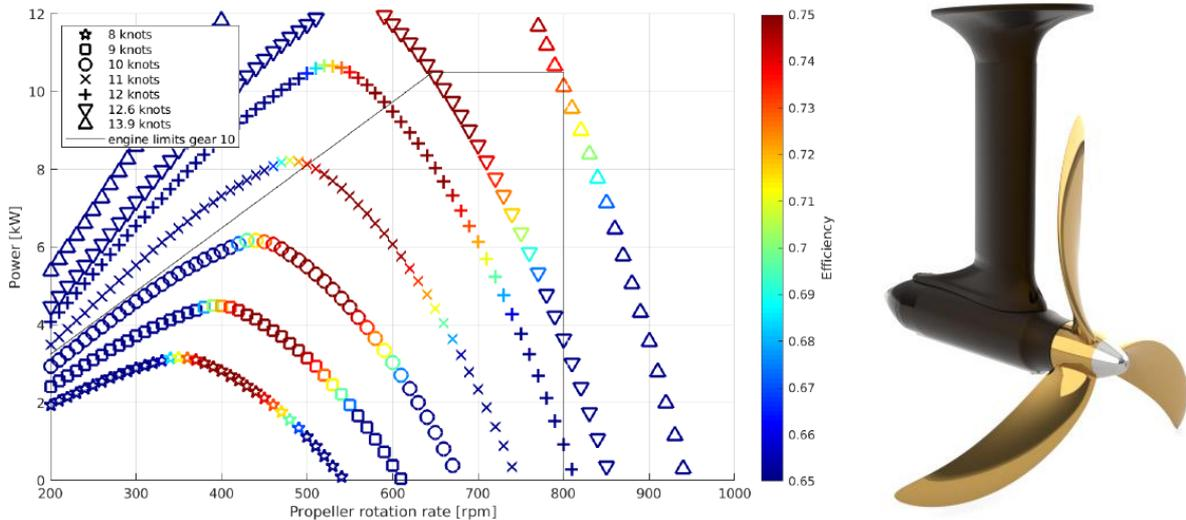
**Figure 5-8:** Left: Propeller curves and engine limits 10.5 kW propeller. Right: Dedicated regeneration system 10.5 kW
