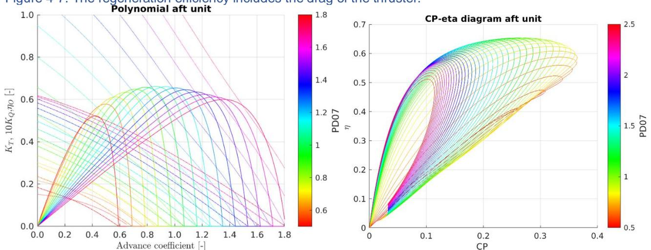
Figure 4-7: Polynomials of performance in propulsion (left) and regeneration (right)
