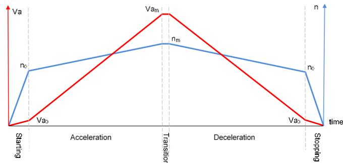
**Figure 5-4:** Trapezoidal variation of advance speed  $V_a$  and rotation rate  $n$  (example only).
