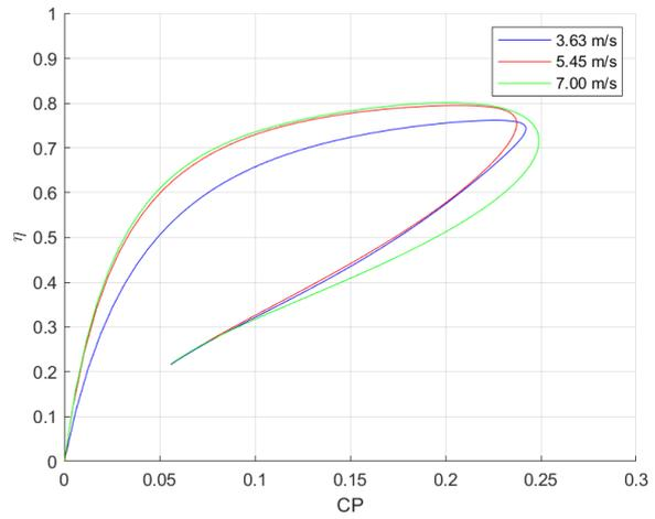
Figure 5-5: Speed dependency on propeller efficiency  $\eta$  and power regeneration  $CP$  at model scale 2.
