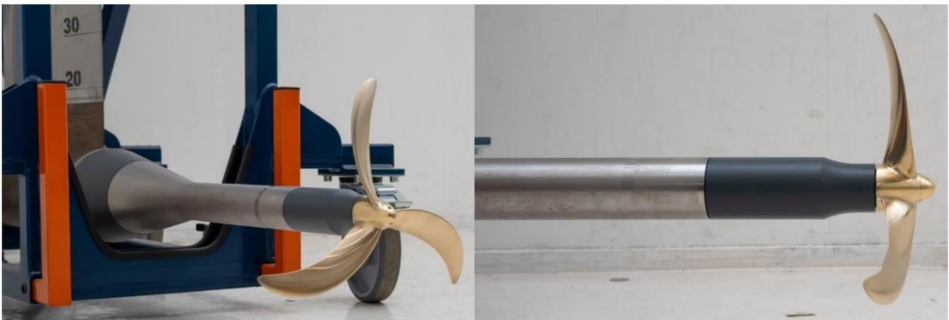
**Figure 5-3:** Photographs of the manufactured propeller, including cap and stream piece.
