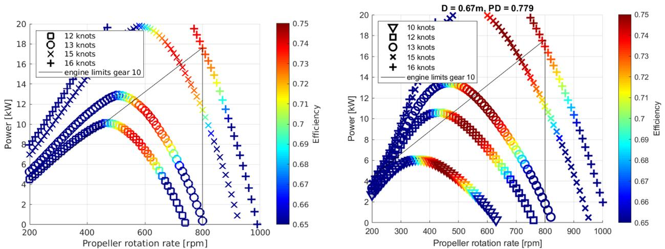
Figure 5-6: Propeller curves and engine limits, computation (left) and measurement (right). Unit efficiency.
