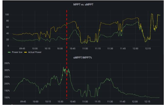
Fig. 12. Test results: a) Comparison of power generation between a traditional optimizer & implementing the string level converter technique b) The aforementioned difference in percentage form. This difference goes up to 300% at the instant of the picture being taken.
