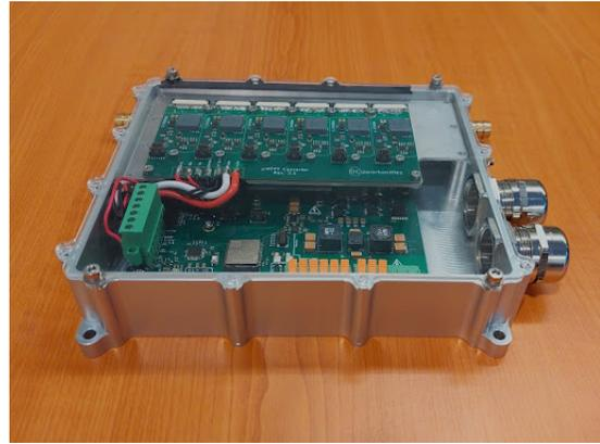
Fig. 9. Physical prototype. The isolated converter is mounted on the lower level and the string level converters are on the top level. The boards are mounted in a watertight metal enclosure.
