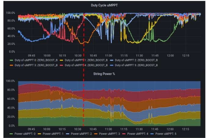
Fig. 11. Test results: a) Duty cycle per string b) Share of total power. When a string is shaded its duty cycle is decreased to maintain the same output current so that the rest of the strings can operate at MPP at 100% duty cycle. When the duty cycle of a string is at its minimum, its contribution to the overall power generation is also minimum.
