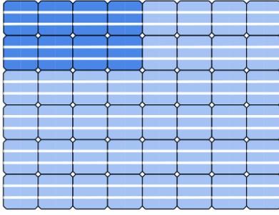
Fig. 1. Drawing of a 48 cell solar panel with one highlighted string. Each string consists of 8 solar cells and each panel consists of 6 strings.
