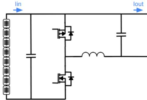
Fig. 3. Low-side-switch step-down converter. Contrary to the conventional step-down converter, this topology utilizes a N-type MOSFET on the low-side switch and a P-type MOSFET on the top-side switch. When the duty cycle is above 50%, the current will flow through the low-side switch most of the time. N type MOSFETs offer better electrical characteristics than P-type MOSFETs.
