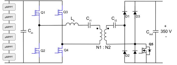
Fig. 5. Schematic of CLLC Isolated Converter.  $C_{r1}$  and  $C_{r2}$  are the resonant series capacitance of the primary and secondary, respectively.  $C_{r2}$  can also be used as a DC blocking capacitor if Q5 is permanently closed. Q1-Q4 are shown in blue because they are 80V rated GaN high electron mobility transistors (HEMTs)
