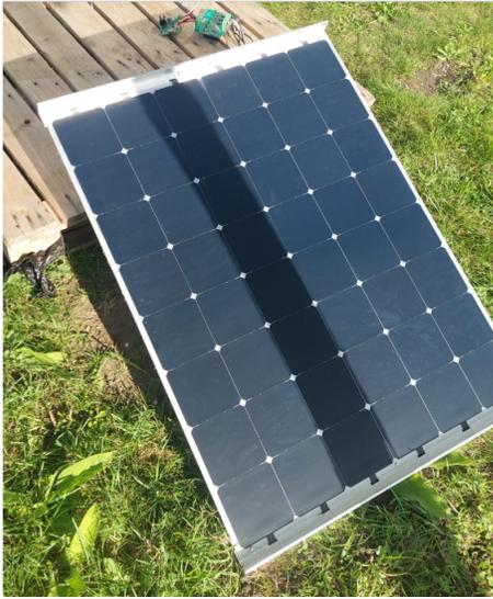
Fig. 10. Testing setup. The photovoltaic panel is placed behind a tree casting a vertical shadow onto it. Each column is composed by a string of 8 cells and at the instant when the picture was taken the 3rd string starting from the left is fully shaded by the tree.
