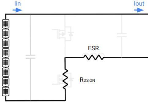
Fig. 4. Current flow at 100% duty cycle. When shading does not occur, switching losses are eliminated and conduction losses occur at the ESR of the inductor and  $R_{ds,on}$  of the N type MOSFET.
