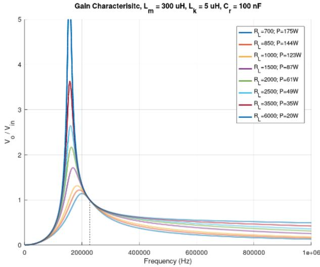
Fig. 6. Gain characteristic of resonant tank where  $f_{r1} = 225kHz$  (labeled with dotted black line). The different color curves show the frequency vs. gain behavior under various load conditions
