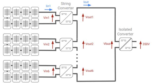
Fig. 2. System Overview Diagram. The system consists of a 2 step conversion. Each string of photovoltaic cells consists of 8 units connected to a string converter. Each system consists of 6 of these and their outputs are connected in series. The second conversion occurs at the isolated converter which connects to the DC grid on the output.
